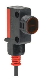
Leuze photoelectric sensor, rectangular, polarized retroreflective, visible red light emission, 0.02-4.5m sensing distance, complementary light-on/dark-on, NPN, 4-wire, pigtail.
