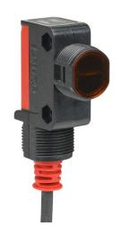
Leuze photoelectric sensor, rectangular, polarized retroreflective, visible red, 0.02-4.5m sensing distance, complementary light-on/dark-on, NPN, 4-wire, 4-pin M12 quick-disconnect.
