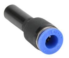
NITRA pneumatic push-to-connect fitting, plug-in reducer, thermoplastic (PBT) body, (1) 5/16in (8mm) plug-in to (1) 6mm push-to-connect. Package of 5.
