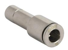
NITRA pneumatic push-to-connect fitting, plug-in reducer, nickel-plated brass body, 5/16in (8mm) plug-in to 6mm push-to-connect. Package of 5.
