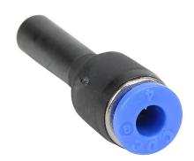
NITRA pneumatic push-to-connect fitting, plug-in reducer, thermoplastic (PBT) body, 6mm plug-in to 5/32in (4mm) tube connection(s). Package of 5.
