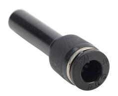
NITRA pneumatic push-to-connect fitting, plug-in reducer, thermoplastic (PBT) body, (1) 5/16in (8mm) plug-in to (1) 1/4in push-to-connect. Package of 5.
