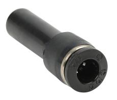
NITRA pneumatic push-to-connect fitting, plug-in reducer, thermoplastic (PBT) body, (1) 3/8in plug-in to (1) 1/4in push-to-connect. Package of 5.
