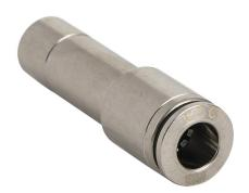
NITRA pneumatic push-to-connect fitting, plug-in reducer, nickel-plated brass body, (1) 3/8in plug-in to (1) 1/4in push-to-connect. Package of 5.
