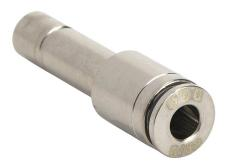
NITRA pneumatic push-to-connect fitting, plug-in reducer, nickelplated brass body, (1) 1/4in plug-in to (1) 5/32in (4mm) push-toconnect. Package of 5.
