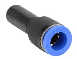
NITRA pneumatic push-to-connect fitting, plug-in reducer, thermoplastic (PBT) body, (1) 12mm plug-in to (1) 10mm push-to-connect. Package of 5.
