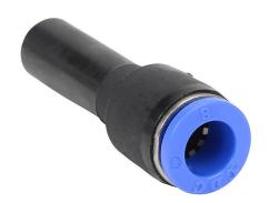
NITRA pneumatic push-to-connect fitting, plug-in reducer, thermoplastic (PBT) body, (1) 10mm plug-in to (1) 5/16in (8mm) push-to-connect. Package of 5.
