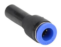
NITRA pneumatic push-to-connect fitting, plug-in reducer, thermoplastic (PBT) body, 10mm plug-in to 5/16in (8mm) tube connection(s). Package of 5.
