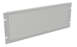
Hammond rack panel, 4U, 19in rack width, flanged, perforated, carbon steel, RAL 7035 light gray, powder coat finish.
