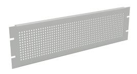
Hammond rack panel, 3U, 19in rack width, flanged, perforated, carbon steel, RAL 7035 light gray, powder coat finish.
