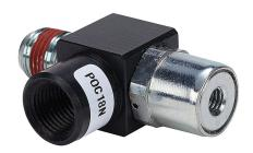
NITRA pneumatic threaded fitting, pilot operated check valve, rotating, anodized aluminum body, zinc-plated brass threads, (1) 1/8in female NPT to (1) 1/8in male NPT to (1) #10-32 female threaded connection(s).
