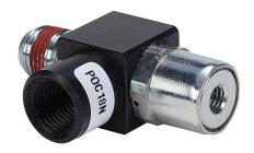
NITRA pneumatic threaded fitting, pilot operated check valve, rotating, anodized aluminum body, zinc-plated brass threads, (1) #10-32 female UNF to (1) 1/8in female NPT to (1) 1/8in male NPT.
