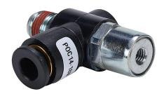
NITRA pneumatic threaded fitting, pilot operated check valve, rotating, anodized aluminum body, zinc-plated brass threads, (1) #10-32 female UNF to (1) 1/4in push-to-connect to (1) 1/8in male NPT.
