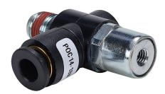
NITRA pneumatic threaded fitting, pilot operated check valve, rotating, anodized aluminum body, zinc-plated brass threads, (1) 1/4in push-to-connect tubing to (1) 1/8in male NPT to (1) #10-32 female threaded connection(s).
