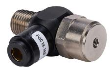
NITRA pneumatic threaded fitting, pilot operated check valve, rotating, anodized aluminum body, nickel-plated brass threads, (1) #10-32 female UNF to (1) 1/4in male NPT to (1) 1/4in push-to-connect.
