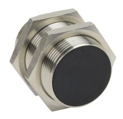
AutomationDirect inductive proximity sensor, tubular, 30mm diameter x 50mm body, bronze-plated brass housing, PNP, N.C. output, 15mm sensing distance, flush, 100 Hz switching frequency, IP65 IP66 IP67 IP68 IP69K, 4-pin M12 quick-disconnect.
