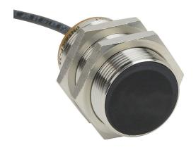
AutomationDirect inductive proximity sensor, tubular, 30mm diameter x 50mm body, bronze-plated brass housing, PNP, N.C. output, 15mm sensing distance, flush, 100 Hz switching frequency, IP65 IP66 IP67 IP68 IP69K, pigtail.
