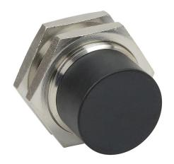
AutomationDirect inductive proximity sensor, tubular, 30mm diameter x 50mm body, bronze-plated brass housing, PNP, N.O. output, 22mm sensing distance, non-flush, 100 Hz switching frequency, IP65 IP66 IP67 IP68 IP69K, 4-pin M12 quick-disconnect.
