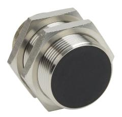
AutomationDirect inductive proximity sensor, tubular, 30mm diameter x 50mm body, bronze-plated brass housing, PNP, N.O. output, 15mm sensing distance, flush, 100 Hz switching frequency, IP65 IP66 IP67 IP68 IP69K, 4-pin M12 quick-disconnect.
