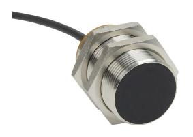
AutomationDirect inductive proximity sensor, tubular, 30mm diameter x 50mm body, bronze-plated brass housing, PNP, N.O. output, 15mm sensing distance, flush, 100 Hz switching frequency, IP65 IP66 IP67 IP68 IP69K, pigtail.
