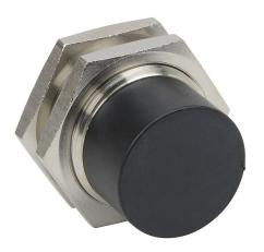
AutomationDirect inductive proximity sensor, tubular, 30mm diameter x 50mm body, bronze-plated brass housing, NPN, N.O. output, 22mm sensing distance, non-flush, 100 Hz switching frequency, IP65 IP66 IP67 IP68 IP69K, 4-pin M12 quick-disconnect.
