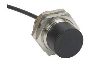
AutomationDirect inductive proximity sensor, tubular, 30mm diameter x 50mm body, bronze-plated brass housing, NPN, N.O. output, 22mm sensing distance, non-flush, 100 Hz switching frequency, IP65 IP66 IP67 IP68 IP69K, pigtail.
