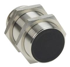
AutomationDirect inductive proximity sensor, tubular, 30mm diameter x 60mm body, bronze-plated brass housing, PNP, N.C. output, 15mm sensing distance, flush, 100 Hz switching frequency, IP65 IP66 IP67 IP68 IP69K, 4-pin M12 quick-disconnect.
