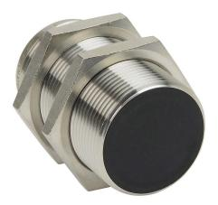
AutomationDirect inductive proximity sensor, tubular, 30mm diameter x 60mm body, bronze-plated brass housing, NPN, N.C. output, 15mm sensing distance, flush, 100 Hz switching frequency, IP65 IP66 IP67 IP68 IP69K, 4-pin M12 quick-disconnect.
