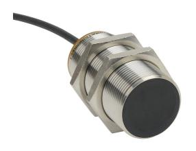
AutomationDirect inductive proximity sensor, tubular, 30mm diameter x 65mm body, bronze-plated brass housing, NPN, N.C. output, 15mm sensing distance, flush, 100 Hz switching frequency, IP65 IP66 IP67 IP68 IP69K, pigtail.
