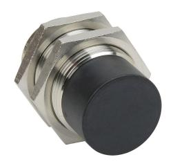
AutomationDirect inductive proximity sensor, tubular, 30mm diameter x 60mm body, bronze-plated brass housing, PNP, N.O. output, 22mm sensing distance, non-flush, 100 Hz switching frequency, IP65 IP66 IP67 IP68 IP69K, 4-pin M12 quick-disconnect.
