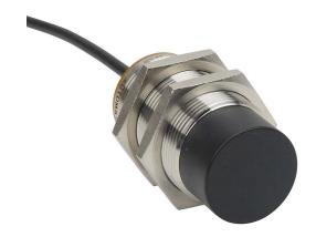
AutomationDirect inductive proximity sensor, tubular, 30mm diameter x 65mm body, bronze-plated brass housing, PNP, N.O. output, 22mm sensing distance, non-flush, 100 Hz switching frequency, IP65 IP66 IP67 IP68 IP69K, pigtail.
