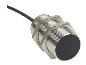
AutomationDirect inductive proximity sensor, tubular, 30mm diameter x 65mm body, bronze-plated brass housing, PNP, N.O. output, 15mm sensing distance, flush, 100 Hz switching frequency, IP65 IP66 IP67 IP68 IP69K, pigtail.
