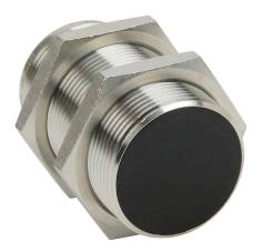
AutomationDirect inductive proximity sensor, tubular, 30mm diameter x 60mm body, bronze-plated brass housing, NPN, N.O. output, 15mm sensing distance, flush, 100 Hz switching frequency, IP65 IP66 IP67 IP68 IP69K, 4-pin M12 quick-disconnect.
