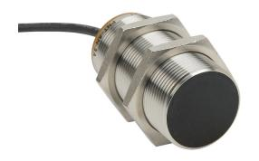
AutomationDirect inductive proximity sensor, tubular, 30mm diameter x 65mm body, bronze-plated brass housing, NPN, N.O. output, 15mm sensing distance, flush, 100 Hz switching frequency, IP65 IP66 IP67 IP68 IP69K, pigtail.
