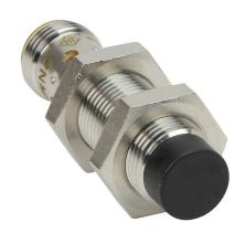
AutomationDirect inductive proximity sensor, tubular, 12mm diameter x 45mm body, bronze-plated brass housing, PNP, N.C. output, 7mm sensing distance, non-flush, 700 Hz switching frequency, IP65 IP66 IP67 IP68 IP69K, 4-pin M12 quick-disconnect.
