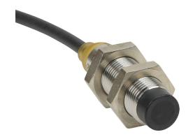
AutomationDirect inductive proximity sensor, tubular, 12mm diameter x 45mm body, bronze-plated brass housing, PNP, N.C. output, 7mm sensing distance, non-flush, 700 Hz switching frequency, IP65 IP66 IP67 IP68 IP69K, pigtail.
