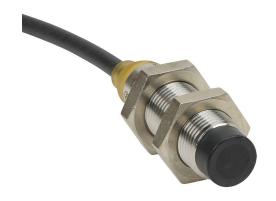
AutomationDirect inductive proximity sensor, tubular, 12mm diameter x 45mm body, bronze-plated brass housing, PNP, N.C. output, 7mm sensing distance, non-flush, 700 Hz switching frequency, IP65 IP66 IP67 IP68 IP69K, pigtail.
