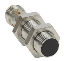
AutomationDirect inductive proximity sensor, tubular, 12mm diameter x 45mm body, bronze-plated brass housing, PNP, N.C. output, 4mm sensing distance, flush, 700 Hz switching frequency, IP65 IP66 IP67 IP68 IP69K, 4-pin M12 quick-disconnect.
