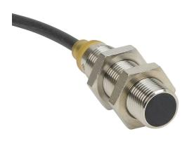
AutomationDirect inductive proximity sensor, tubular, 12mm diameter x 45mm body, bronze-plated brass housing, PNP, N.C. output, 4mm sensing distance, flush, 700 Hz switching frequency, IP65 IP66 IP67 IP68 IP69K, pigtail.
