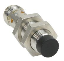
AutomationDirect inductive proximity sensor, tubular, 12mm diameter x 45mm body, bronze-plated brass housing, NPN, N.C. output, 7mm sensing distance, non-flush, 700 Hz switching frequency, IP65 IP66 IP67 IP68 IP69K, 4-pin M12 quick-disconnect.
