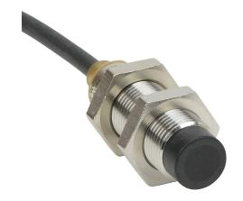
AutomationDirect inductive proximity sensor, tubular, 12mm diameter x 45mm body, bronze-plated brass housing, NPN, N.C. output, 7mm sensing distance, non-flush, 700 Hz switching frequency, IP65 IP66 IP67 IP68 IP69K, pigtail.
