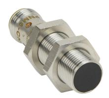
AutomationDirect inductive proximity sensor, tubular, 12mm diameter x 45mm body, bronze-plated brass housing, NPN, N.C. output, 4mm sensing distance, flush, 700 Hz switching frequency, IP65 IP66 IP67 IP68 IP69K, 4-pin M12 quick-disconnect.
