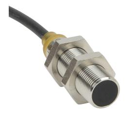
AutomationDirect inductive proximity sensor, tubular, 12mm diameter x 45mm body, bronze-plated brass housing, NPN, N.C. output, 4mm sensing distance, flush, 700 Hz switching frequency, IP65 IP66 IP67 IP68 IP69K, pigtail.
