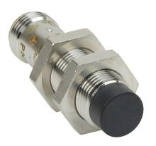
AutomationDirect inductive proximity sensor, tubular, 12mm diameter x 45mm body, bronze-plated brass housing, PNP, N.O. output, 7mm sensing distance, non-flush, 700 Hz switching frequency, IP65 IP66 IP67 IP68 IP69K, 4-pin M12 quick-disconnect.
