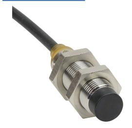
AutomationDirect inductive proximity sensor, tubular, 12mm diameter x 45mm body, bronze-plated brass housing, PNP, N.O. output, 7mm sensing distance, non-flush, 700 Hz switching frequency, IP65 IP66 IP67 IP68 IP69K, pigtail.
