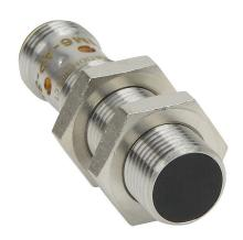
AutomationDirect inductive proximity sensor, tubular, 12mm diameter x 45mm body, bronze-plated brass housing, PNP, N.O. output, 4mm sensing distance, flush, 700 Hz switching frequency, IP65 IP66 IP67 IP68 IP69K, 4-pin M12 quick-disconnect.
