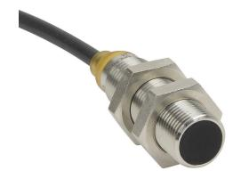
AutomationDirect inductive proximity sensor, tubular, 12mm diameter x 45mm body, bronze-plated brass housing, PNP, N.O. output, 4mm sensing distance, flush, 700 Hz switching frequency, IP65 IP66 IP67 IP68 IP69K, pigtail.
