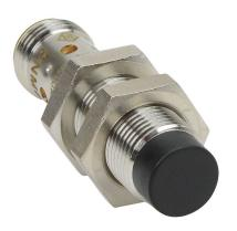
AutomationDirect inductive proximity sensor, tubular, 12mm diameter x 45mm body, bronze-plated brass housing, NPN, N.O. output, 7mm sensing distance, non-flush, 700 Hz switching frequency, IP65 IP66 IP67 IP68 IP69K, 4-pin M12 quick-disconnect.
