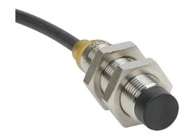
AutomationDirect inductive proximity sensor, tubular, 12mm diameter x 45mm body, bronze-plated brass housing, NPN, N.O. output, 7mm sensing distance, non-flush, 700 Hz switching frequency, IP65 IP66 IP67 IP68 IP69K, pigtail.
