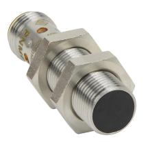
AutomationDirect inductive proximity sensor, tubular, 12mm diameter x 45mm body, bronze-plated brass housing, NPN, N.O. output, 4mm sensing distance, flush, 700 Hz switching frequency, IP65 IP66 IP67 IP68 IP69K, 4-pin M12 quick-disconnect.
