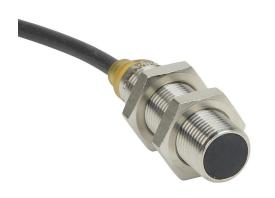
AutomationDirect inductive proximity sensor, tubular, 12mm diameter x 45mm body, bronze-plated brass housing, NPN, N.O. output, 4mm sensing distance, flush, 700 Hz switching frequency, IP65 IP66 IP67 IP68 IP69K, pigtail.
