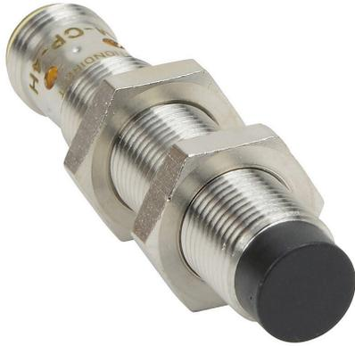
AutomationDirect inductive proximity sensor, tubular, 12mm diameter x 60mm body, bronze-plated brass housing, PNP, N.C. output, 7mm sensing distance, non-flush, 700 Hz switching frequency, IP65 IP66 IP67 IP68 IP69K, 4-pin M12 quick-disconnect.
