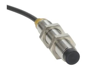
AutomationDirect inductive proximity sensor, tubular, 12mm diameter x 65mm body, bronze-plated brass housing, PNP, N.C. output, 7mm sensing distance, non-flush, 700 Hz switching frequency, IP65 IP66 IP67 IP68 IP69K, pigtail.
