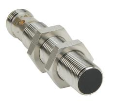
AutomationDirect inductive proximity sensor, tubular, 12mm diameter x 60mm body, bronze-plated brass housing, PNP, N.C. output, 4mm sensing distance, flush, 700 Hz switching frequency, IP65 IP66 IP67 IP68 IP69K, 4-pin M12 quick-disconnect.
